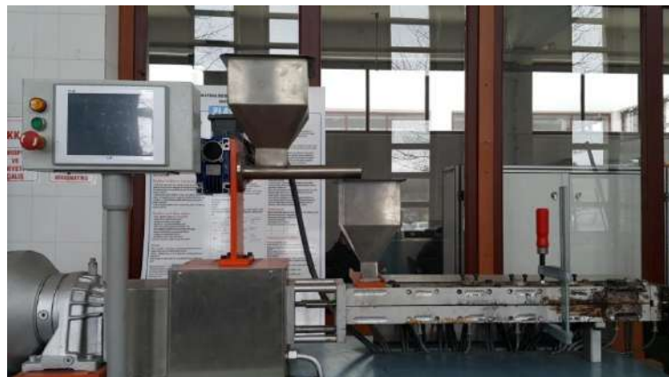
Figure 1. Twin screw extruder utilized in this study
