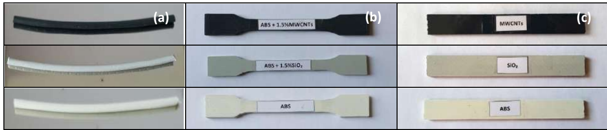
Figure 3. a) Produced filaments, b) Tensile test samples, c) Bending test samples for MWCNT, SiO 2 , ABS.
